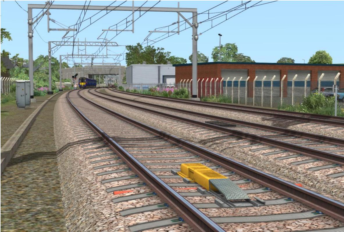
AWS is provided to give train drivers in-cab warnings on the approach to signals, reductions in permissible speed and temporary/emergency speed restrictions, and to apply the brakes in the event that a driver does not acknowledge cautionary warnings given by the system.
