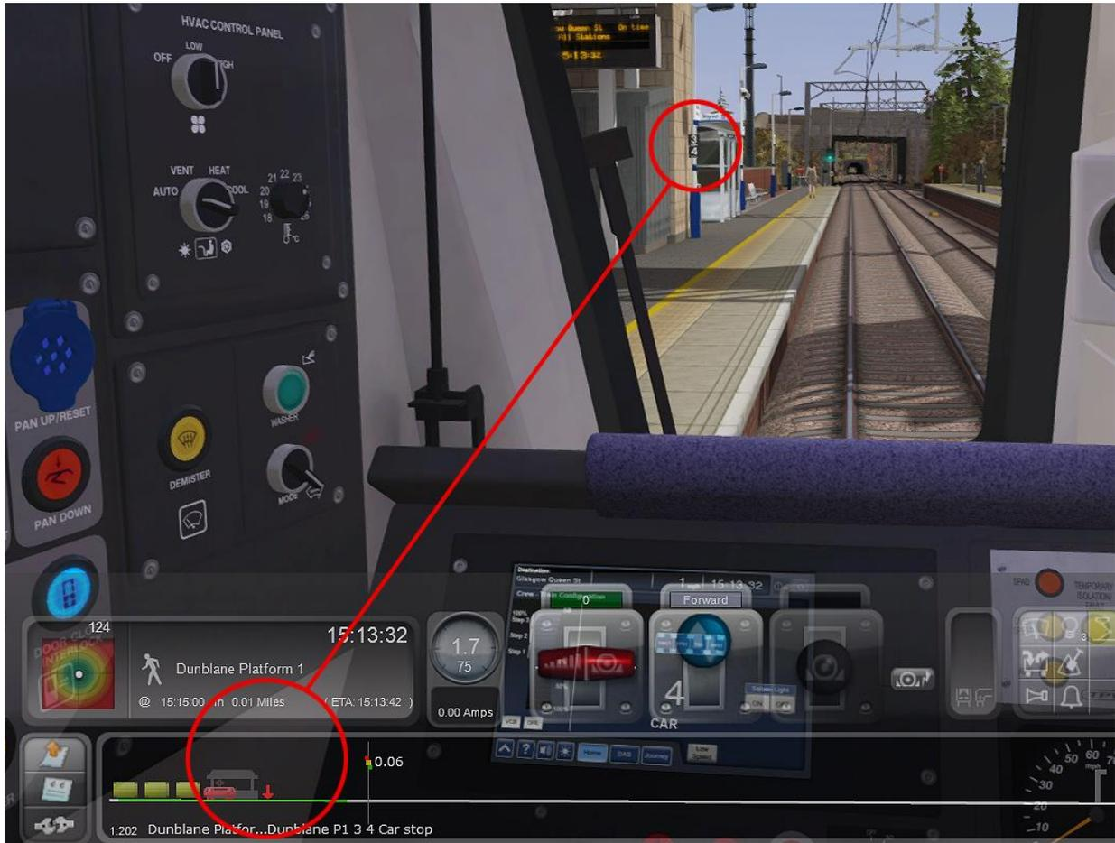
Dynamic stopping points are provided at some station stops and during reversing maneuvers. These trackside signs designate the point where you should stop your train based on the number of vehicles in your consist. The correct stopping point is also indicated on the F4 HUD using a red arrow as shown above.
